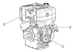
4. Fill the engine oil as per specifications to the maximum mark on the dipstick (E).
