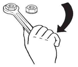
Check and if necessary tighten screws and nuts.
