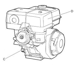
4. Fill the engine oil to the maximum mark on the dipstick (C).
