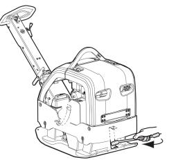
• Check the screws and nuts on the safety straps, if necessary tighten or replace.
