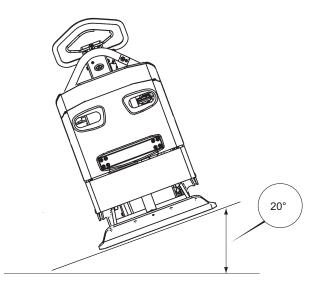
The tilting angle is measured on a hard level surface with the machine stationary. Vibration switched OFF and all tanks full.
