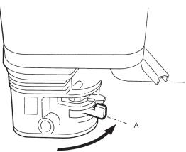
2. Move the throttle control handle to half throttle, position (B).
