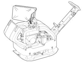
4. Never overfill the tank. Due to the movement of the fuel within the tank, it is possible to have fuel at a higher level than the tank cap, which can lead to a spillage of fuel if the tank cap is opened. This can be avoided by only opening the tank cap when the machine is tilted and the tank cap is at the fuel tank's highest point.
